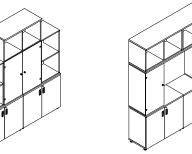
4nos. - Display Box-Double Unit 2nos. - Display Box-Double Unit 2nos. - Display Box-Double Unit with Glass Door 1no. - Top Ledge L-900 2nos. - Top Ledge L-1800
